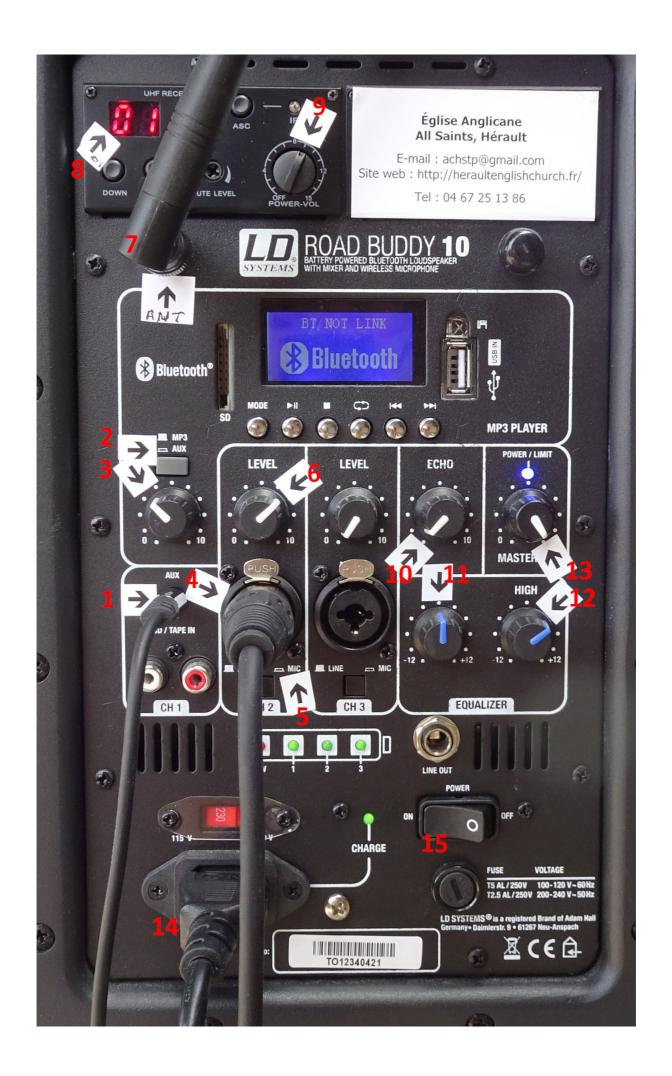
9 The radio headset microphone takes two AA batteries and these do not last long, only two or three services. There is a battery tester (see photo): please check the batteries before each use. The battery compartment of the microphone unit is accessed at the bottom, with OPEN and CLOSED in black and rather difficult to see. The correct way up for the batteries is shown in a similar way on the side with the clip.
