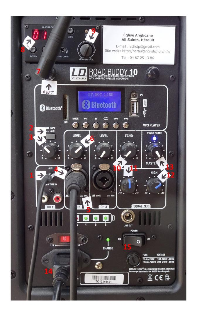
14 Plug the mains lead in if power is available. This type of power cord is notorious for coming loose, so check that it is pushed fully home. If you are in the temple at St Pargoire and there is no mains power, check that the power in the building is still on. The circuits there are very limited and can manage only two power-hungry appliances, eg the coffee urn and one kettle. The MCB trip to restore power is in the lavatory area above the sink.
