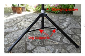
Slide the top of the stand out and insert the metal peg into the third hole from the top (there are some marks next to this) and tighten the clamping screw.
