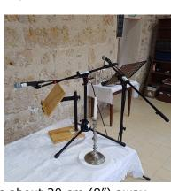
wall as the stand will allow and in front of the microphones to avoid feedback. The reading desk and microphones are best on the kitchen door side of the altar to give maximum distance from the amplifier.
